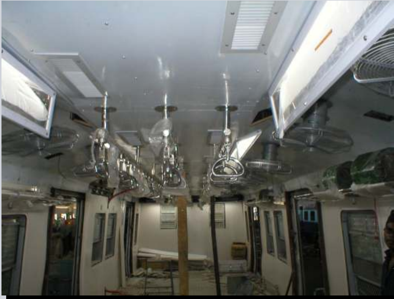
Car interiors – Ventilation system, fans, lights
