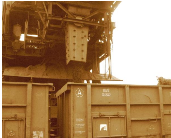
Figure 4: Moveable wagon loader in operation at Megahataburu
