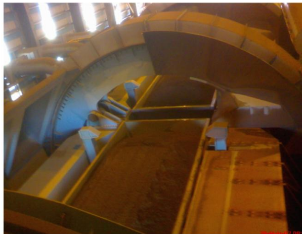
Figure 5: Rotary coupler ore cars on the dumper in Pilbara Railway, Australia
